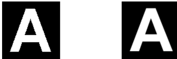
Figure 8 – Antialiasing (the character on the right is antialiased)
